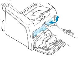
3 With a dry lint-free cloth, wipe away any dust and spilled toner from the toner cartridge area and the toner cartridge cavity.
